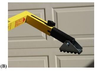
10. (A) Pull stationary hook through inside of ladder first, then (B) position the slide hook to proper width to accommodate the width needed to grab the rail of the ladder. Tighten both plastic wing screws firmly to lock device into place. In the event that a ladder rung is in the way, install the device below the rung even though it will then not be completely flush with the back side of the ladder rails. Be sure that all four plastic wing screws are tightened firmly. (See pictures below)
