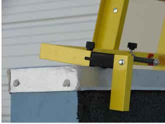
(A) Slide parapet wall extensions back toward ladder until legs stop against or "bite" the back side of the wall, locking device to parapet. (B) Then, tighten both wing screws. (See
