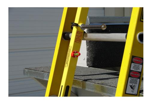
7. Hold Safe T Climb device to the either hand, again gripping at center of device with hooks facing toward you, and carefully proceed up ladder. Maintain three point contact with ladder while climbing. If possible have someone (foot the ladder) at the bottom while climbing. The person footing the ladder should maintain visual contact with the climber in the event that the unit was dropped by the climber. (See pictures below)
