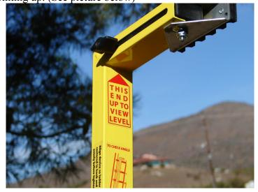
**5**. Facing ladder, place Safe T Climb device vertically against rungs of ladder to verify proper angle for climbing. See the "To Check Angle" label. (See picture below)
