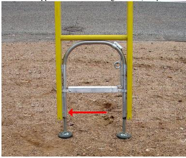
Extend ladder, ensuring that the ladder reaches three feet above the roofline. (The space between rungs is 12 inches on all ladders.) (See pictures below)
